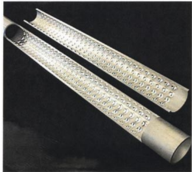
Fig. 1 Sample test channel with machined concavities
